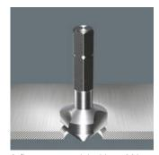
3-flute countersink bits, 90° • Application: Deburring, chamfering and countersinking • ½" drive suitable for holders as per DIN 3126-D 6.3 (ISO 1173) • Hexagon shaft for very high torque transfer • HSS = high speed steel • Finely adjusted material elasticity for long service life • 3 tips • Excellent centring properties • Straightforward cutting • Perfect chip removal • Low jamming risk • Precise return control • High corrosion protection
